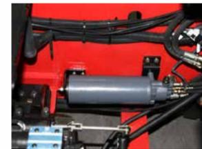
There's an energy accumulator applied in the braking system, which means when the engine is shut down, it can also provides more than 4 times emergency brake.
